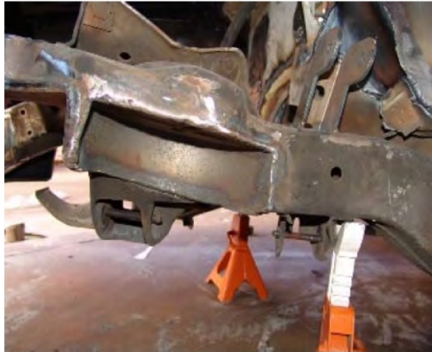
Driver side with control arms and spindles removed. Shown with SPRING POCKET ELIMINATORS & SHOCK RELOCATOR.
